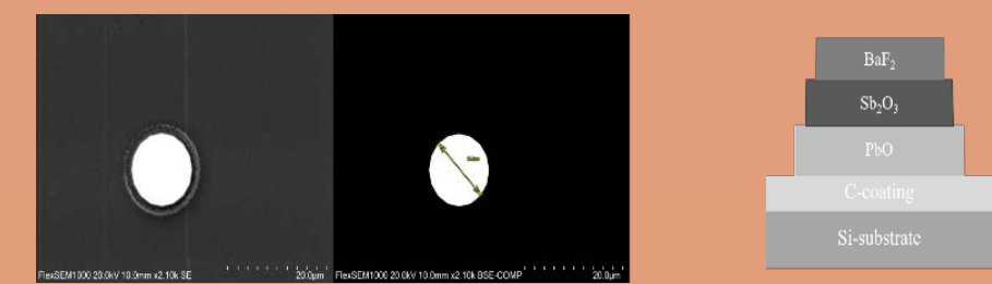
Figure 2 shows the image of synthetic GSR particle of PT sample by using SEM in secondary electron and backscattered electron mode (Left) and the schematic cross-section of PT sample (Right).
