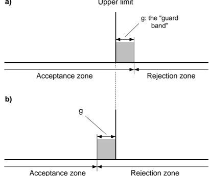
Figure 2: Acceptance and Rejection zones for an Upper Limita)Upper limit
