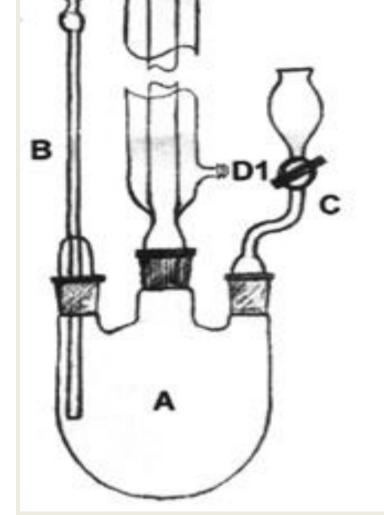
A- Round bottomed three neck flask, 500 mL B- Opened tube with two top bulbs C- Funnel with tap D - Liebig condenser D1 - Water entrance D2 - Water exit E - Spherical socket joints F- Absorption tube containing the NaOH solution G - Tube joint H - Head of the second absorption tube with a tube for CS<sub>2</sub> spread through the colour reagent I - Absorption tube containing the colour reagent J- Connection to the vacuum system.
