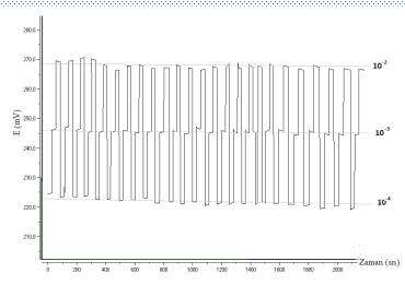
Repeatability of the obtained Ca<sup>2+</sup> - selective microelectrode
